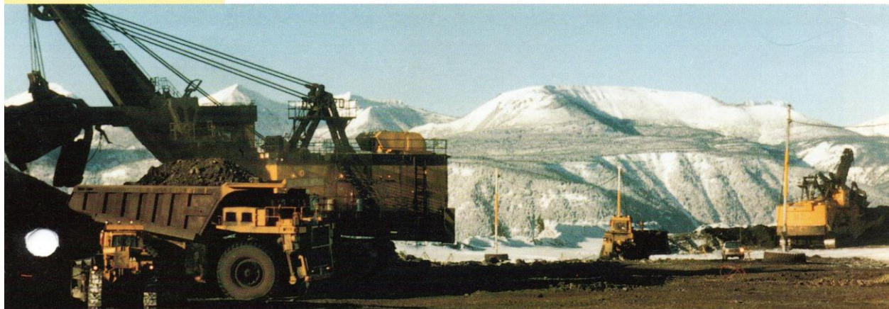
Working The Same Bank — One of the original P&H Mark I 2800 shovels (right background) digs in the same bank as the mine's latest P&H 4100A shovel.
